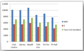
2015 yielded higher values for energy, revenue generation and tons of CO2 avoided when compared with 2014. The chart at left demonstrates this comparison and shows totals over the life of the system so far.
