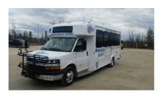
Bike racks allow transit customers to bicycle to transit stops, mount their bicycle on one of two bike mounts then board the bus. At the end of a trip, the bicyclist can then continue travel. Doing so expands the transit market potential and is a step towards a
